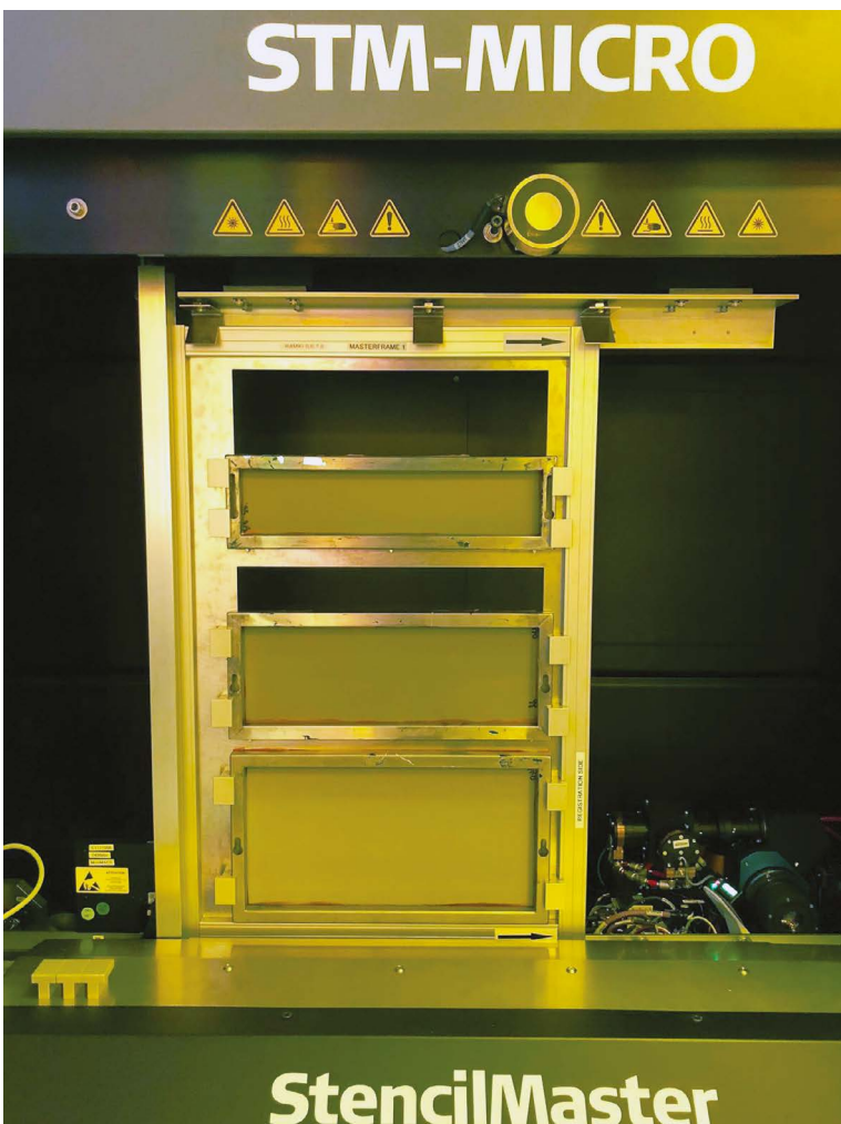
Several small frames can be edited in one step using the masterframe option from SignTronic and Grünig.
