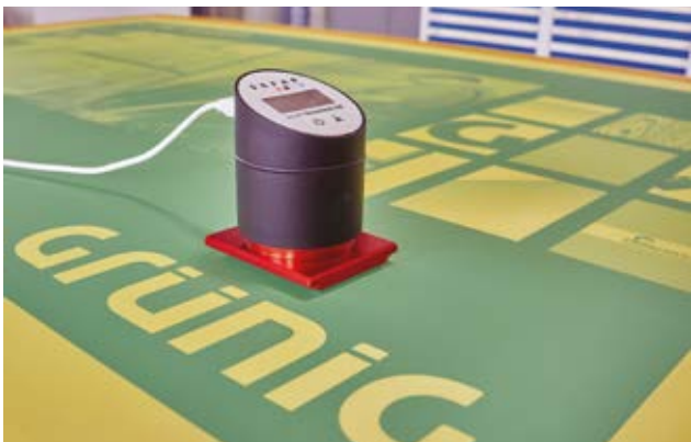
Measuring of the mesh tension with the Tensocheck100 from SEFAR.
